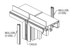
SLIDE FRAMES TOGETHER AND APPLY INSIDE MULLION. APPLY CAULK ALONG JOINT BETWEEN FRAMES AND APPLY OUTSIDE MULLION.
