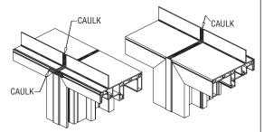
IMPORTANT: USE A QUALITY EXTERIOR GRADE SILICONE CAULK. APPLY 1/4" BEAD OF CAULK ACROSS THE HEAD OF BOTH FRAMES, AS SHOWN, BEFORE APPLYING THE DRIP CAP - APPROXIMATELY 1/4" AWAY FROM THE OUTSIDE EDGE OF THE FRAME. APPLY CAULK ACROSS THE ENDS OF THE FRAMES AND UP THE FINS. BE SURE THE ENTIRE WIDTH OF THE GAP IS COVERED AND THAT CAULK OVERLAPS BOTH FRAMES BY AT LEAST 1/2".
