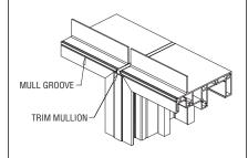
TRIM OUTSIDE MULLION EVEN WITH MULL GROOVE AT THE TOP, TO ALLOW DRIP CAP TO BE INSTALLED, AND EVEN WITH SILL AT THE BOTTOM.
