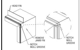
REMOVE NAILING FINS FROM THE JAMBS BEING MULLED TOGETHER. NOTCH MULLION GROOVE FOR THE DRIP CAP. IF APPLICABLE, REMOVE THE J-CHANNEL AS WELL.
