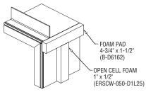
APPLY ONE FOAM PAD (HORIZONTALLY) AT THE TOP AND BOTTOM, AS SHOWN.
